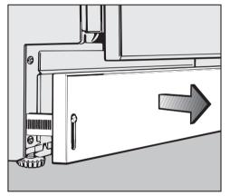
Screw the toekick onto the installed brackets, with the cutting lines towards the top, and pull out evenly until it aligns with the toekick of the adjoining cabinets.
